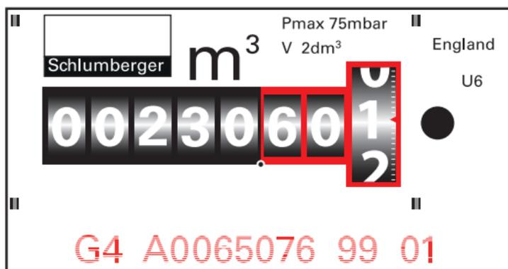
To gas rate a metric meter, note the first reading and run the appliance for 2 minutes (see Note) the end of which you take the second reading. Subtract the first reading from the second to establish the amount of gas used.
